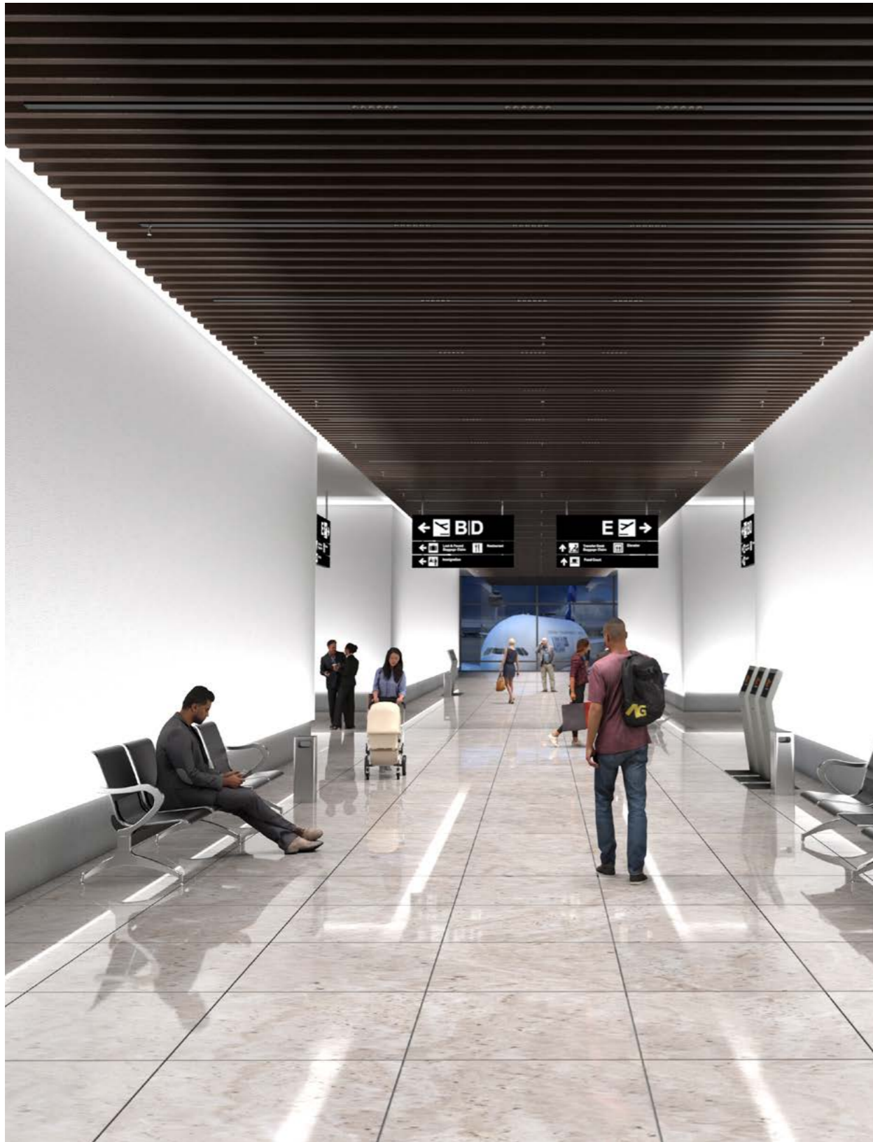
Beam angle Narrow 15°x65° Wall surfaces invisibly illuminated from the floor
